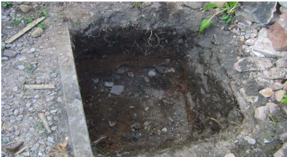
Photograph No 2 Trial Hole 600mm x 600mm x 600mm deep 300mm black top soil underlain with light brown medium coarse sand interspersed with rounded gravel sized 25mm to 50mm
