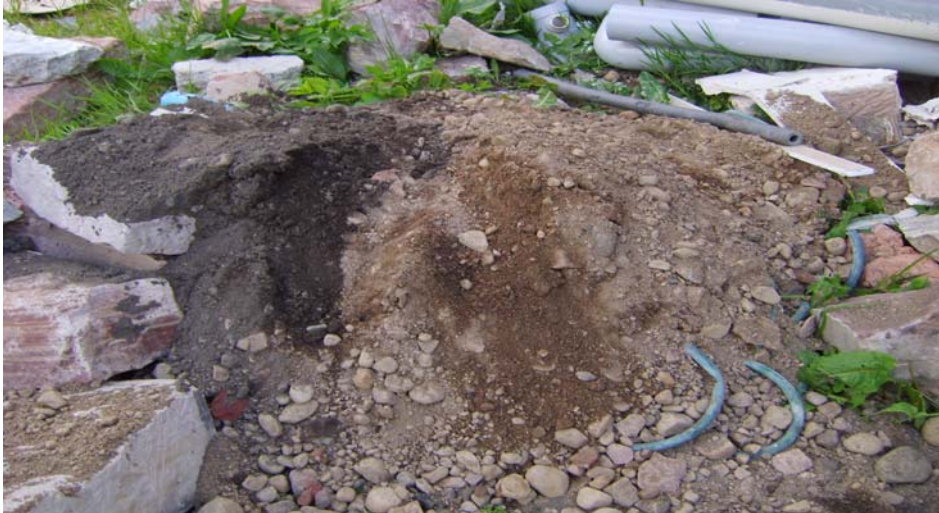
Photograph No 3 Spoil From Trial Hole Showing black top soil and light brown medium coarse sand interspersed with rounded gravel sized 25mm to 50mm
