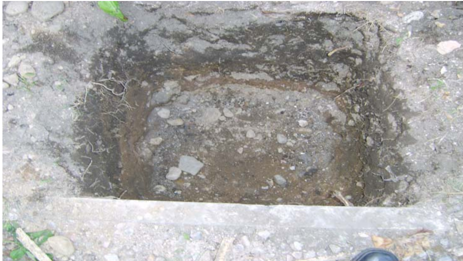
Photograph No 1 Trial Hole 600mm x 600mm x 600mm deep 300mm black top soil underlain with light brown medium coarse sand interspersed with rounded gravel sized 25mm to 50mm
