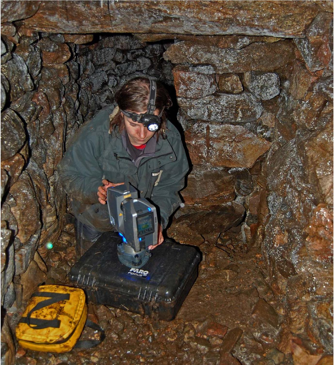
**Illus 2a:** the site during survey (using Faro Focus 3D laser scanner)
